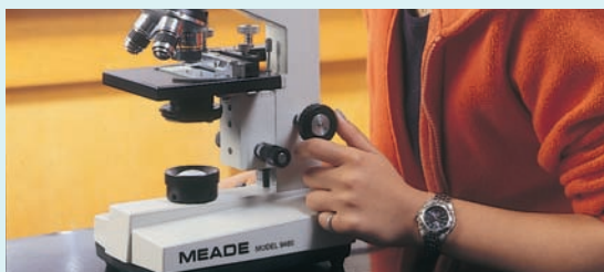
Figure 1.7 The coarse adjustment knob moves the stage up or down.
