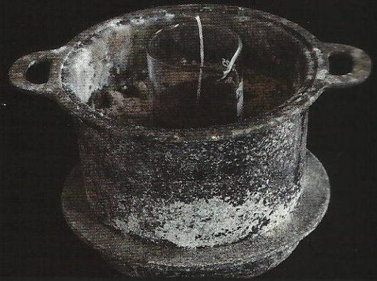
1 Powdered iron oxide and aluminum are mixed in a glass beaker. As a precaution, the beaker is placed in a cast-iron vessel filled with sand. It's a dangerous combination!
